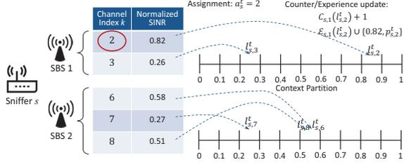
Fig. 4: Context partition and counter/experience update. Sniffer  $s$  have 5 channels in  $\mathcal{C}_s^t$  with  $\{2, 3\}$  operated by SBS 1 and  $\{6, 7, 8\}$  operated by SBS 2. The illustration assumes sniffer  $s$  is assigned to channel 2 and the observed non-outage fraction is  $p_{s,2}^t$ .
