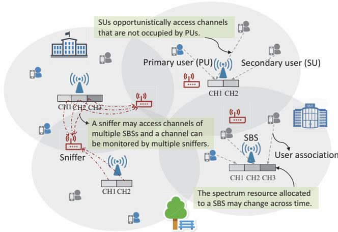
Fig. 1: Passive monitoring system for SCRN. The gray rectangles represent the channels operated by SBSs, which vary over time; a red dash line indicates that a channel can be monitored by a sniffer.
