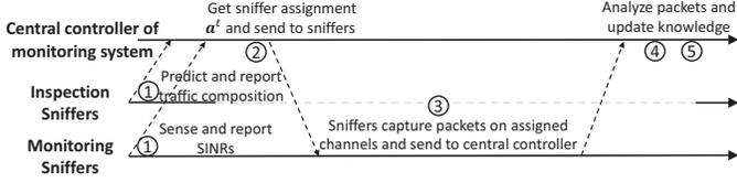
Fig. 3: Time diagram for the SCA problem with OSA.
