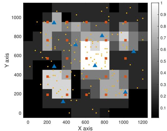
Fig. 5: Deployment of SBSs, sniffers, and users. The background color is the user population density; the blue triangles are SBSs, red squares are sniffers, yellow circles are users in a time slot.
