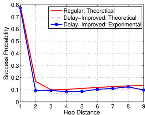
Fig. 20. Success probability under delay-improved greedy routing (14.5% inference error, 20% communication and 40% social link failure).
