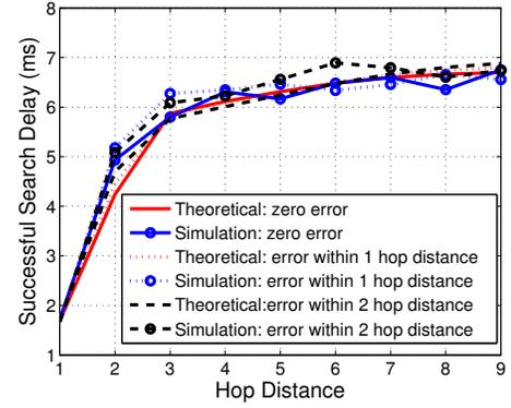
Fig. 14. Delivery delay with distance estimation errors.
