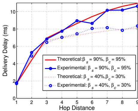
Fig. 18. Measurements of delivery delay with different communication and social link failures.
