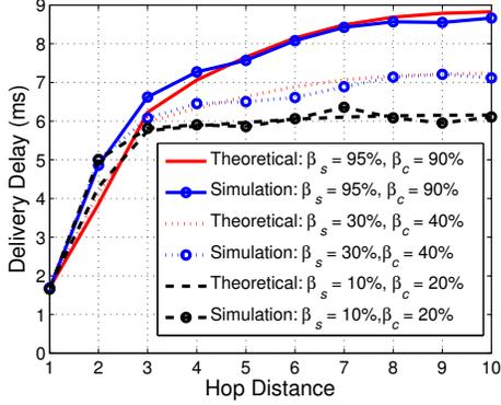
Fig. 10. Average delivery delay with different communication and social link failures.
