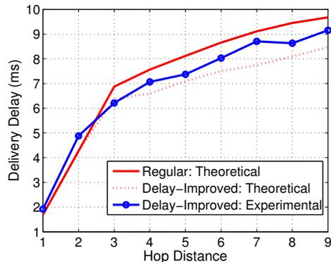
Fig. 19. Delivery delay under delay-improved greedy routing (14.5% inference error, 20% communication and 40% social link failure).
