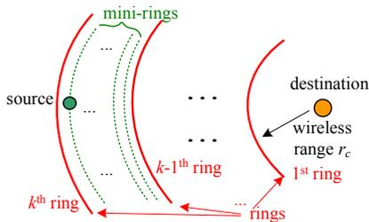
Fig. 3. The source-destination distance divided by rings and mini-rings.
