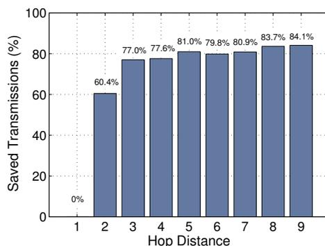
Fig. 23. Percentage of saved transmissions in energy-saving greedy routing (20% communication and 40% social link failure).
