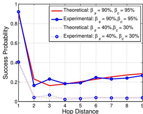
Fig. 17. Measurements of success probability with different communication and social link failures.
