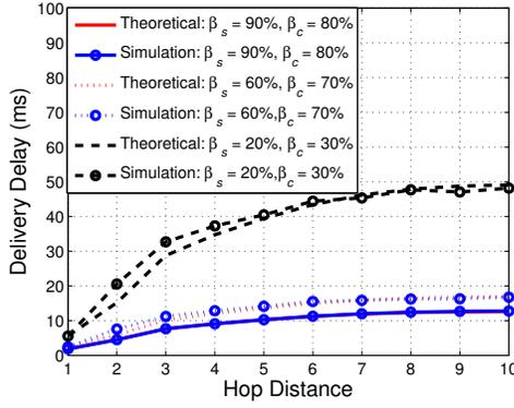
Fig. 12. Average delivery delay under persistent transmission with different communication and social link failures.
