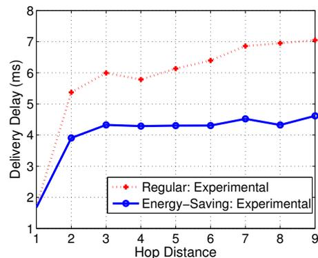
Fig. 22. Comparison of delivery delay under regular greedy routing and energy-saving greedy routing (20% communication and 40% social link failure).
