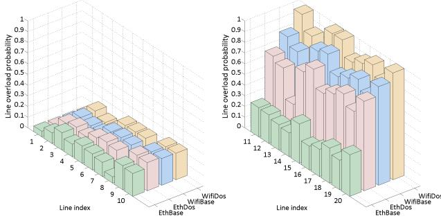
Fig. 10. Line failure probability for IEEE 14-bus system.
