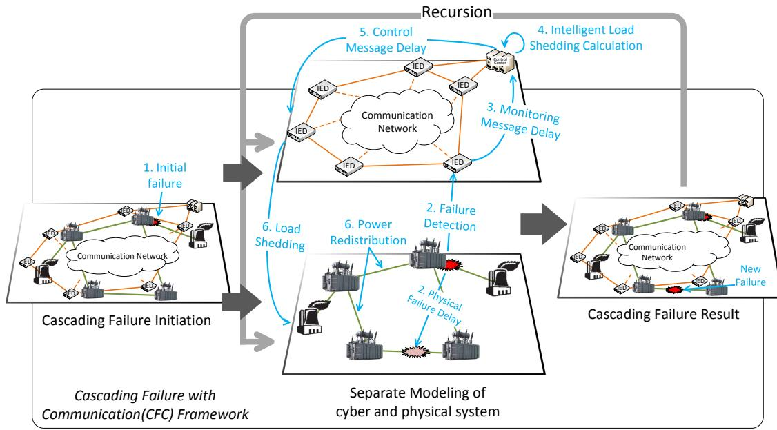
Fig. 3. The Cascading Failure with Communication (CFC) framework.
