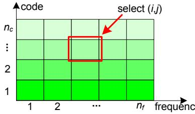
Fig. 1.  $N_f$  frequency and  $N_c$  code channels available.
