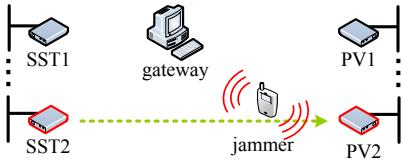
Fig. 8. Attack scenario in the anti-islanding network.
