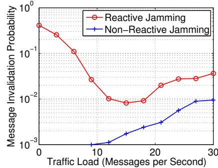
Fig. 10. Coordinated: Message invalidation probability versus traffic load.
