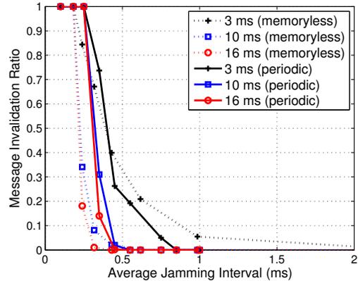
Fig. 10. The message invalidation ratios of GOOSE applications under non-reactive jamming.
