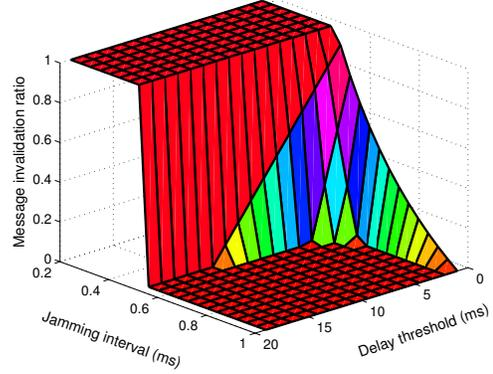
Fig. 8. The message invalidation ratio for a time-critical application under non-reactive periodic jamming.
