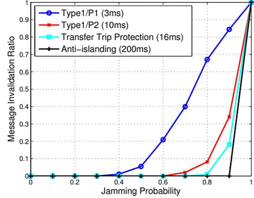
Fig. 9. The message invalidation ratios of four different GOOSE applications under reactive jamming.
