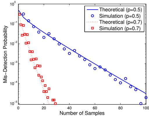
Fig. 11. Theoretical mis-detection probability ( $1 - P_D$ ) versus simulated mis-detection probability. The threshold  $p^*$  is set to be 0.3. The jammer has two probabilities:  $p = 0.5$  and  $p = 0.7$ .
