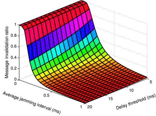
Fig. 7. The message invalidation ratio for a time-critical application under non-reactive memoryless jamming.
