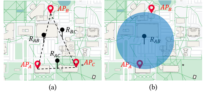
Figure 3: LLT inference attack: (a) The geographic locations of AP_A , AP_B , and AP_C in LLT calculated using the position estimates R_{AB} , R_{BC} , and R_{AC} from API requests with pairwise APs, i.e., (AP_A, AP_B) , (AP_B, AP_C) , and (AP_A, AP_C) using the range-free mode and (b) AP_A and AP_B lie on the circle around the position estimate R_{AB} given the accuracy field.
