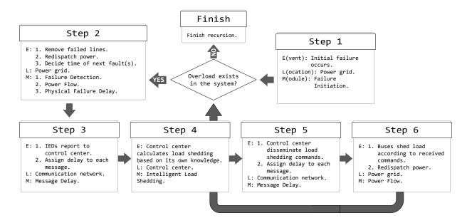
Fig. 4. Simulation Sequence in Each Iteration.
