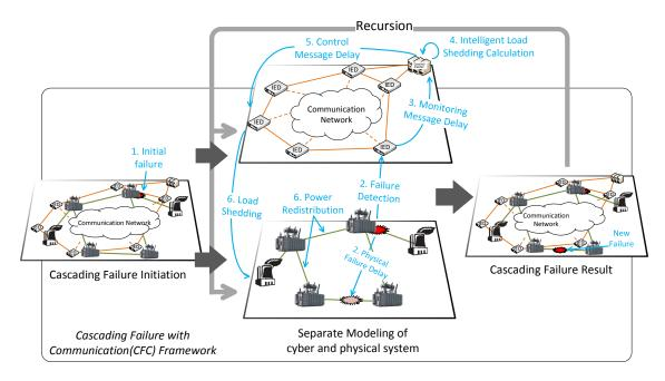
Fig. 3. The Cascading Failure with Communication (CFC) framework.
