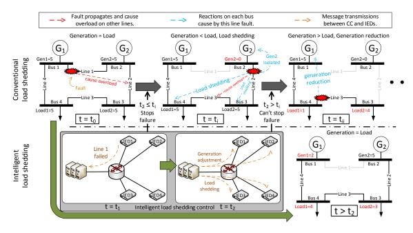
Fig. 2. Cascading failures in conventional power grid, and communication-assisted smart power grid.
