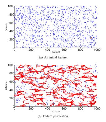
Fig. 9. An initial failure explodes to the entire network.
