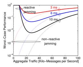
Fig. 3. Coordinated communication: worst-case delay performance  $\mathbb{P}(D_k > \sigma)$  versus aggregate traffic  $\gamma_k$  at node k for time-critical applications with delay thresholds of 3–9ms.  $(N_f=N_c=10, T_L=1\text{ms}, \rho=0.1, \text{ and } \tau=1\mu\text{s.})$
