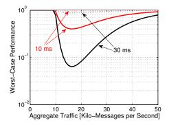
Fig. 5. Uncoordinated communication: worst-case  $\mathbb{P}(D_k > \sigma)$  versus  $\gamma_k$  with delay thresholds of 10ms and 30ms. ( $N_f$ =10,  $N_c$ =2,  $T_L$ =1ms,  $\rho$ =0.1, and  $\tau$ =1 $\mu$ s.)
