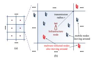
Fig. 1. Network architecture: infrastructure nodes and mobile nodes.
