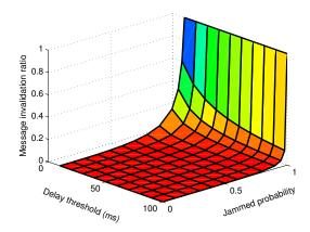
Fig. 4. Upper bound of message invalidation ratio for a time-critical application with 10ms $<\sigma<$ 100ms, 0<p<1,  $N_{\rm mac}$ =3, and  $\mathbb{E}(d_i)$ = 1ms.
