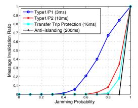
Fig. 7. The message invalidation ratios of four different GOOSE applications.
