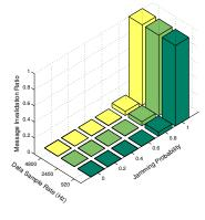
Message invalidation ratio (Type-1A/P1 GOOSE with 3ms limit) as a function of jamming probability p as a function of jamming probability pand transmission rate of the MU IED. and transmission rate of the MU IED.
